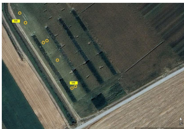
Figure 1. Experimental design – orange dots indicate the location of collecting wind erosion residue. Yellow rectangles show the location of meto stations
