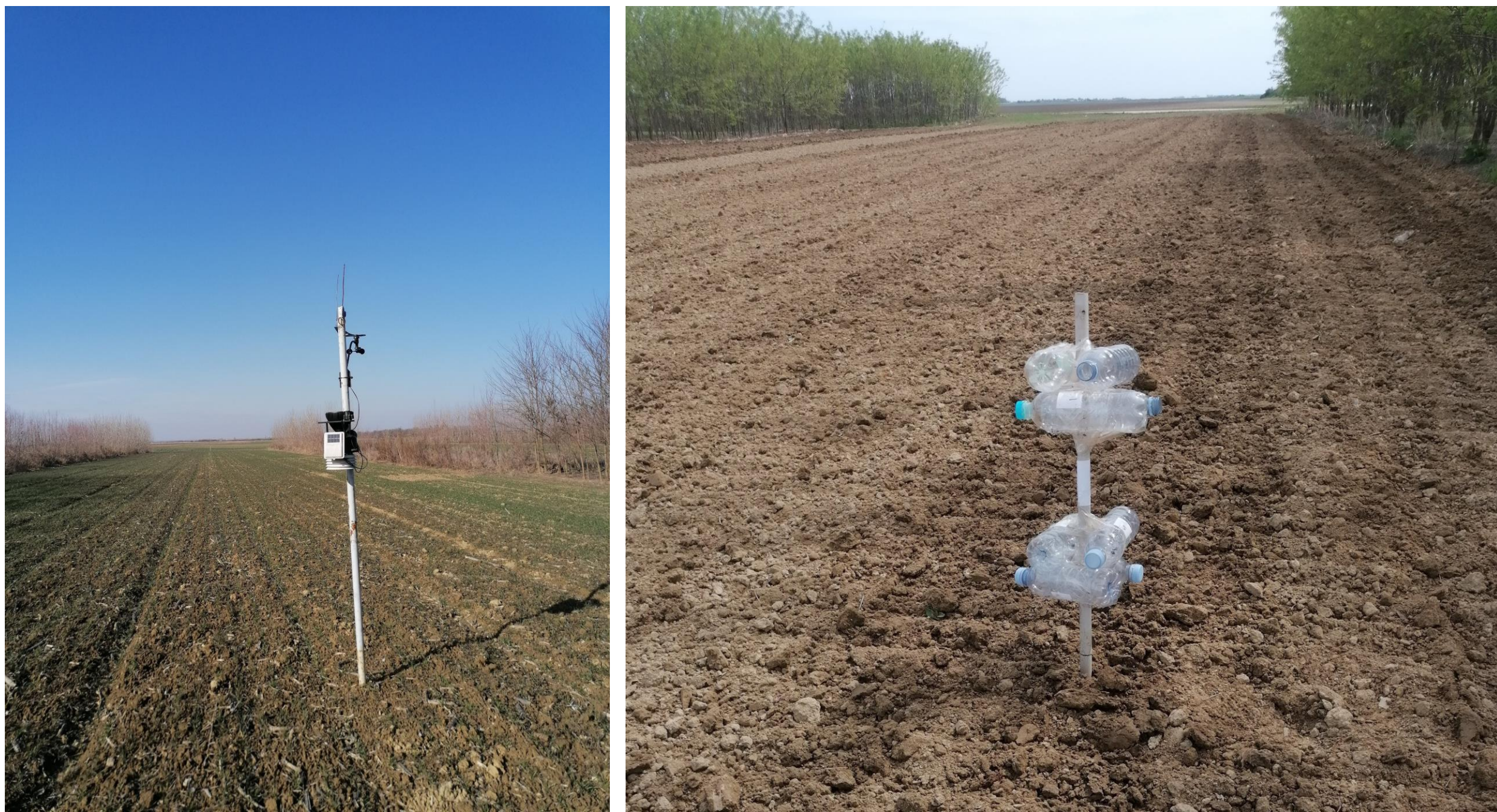
Picture 2 – Meto station and improvised „dust catcher” made out of plastic bottles.
